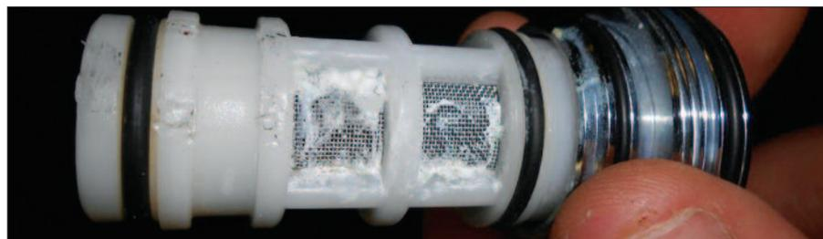
*A TMV strainer with pipe joining compound, Boss White, accumulated on strainer mesh. Pseudomonas aeruginosa was recovered from this TMV strainer and many others within this particular system.*
